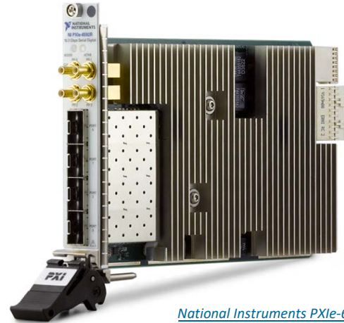
National Instruments PXIe-6592 card
