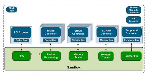
> The user sandbox (in green) provides easy access to optimized interfaces and ample debug capabilities.
