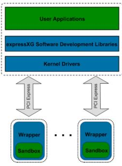
> The interface wrapper is delivered as a synthesized netlist, while the sandbox is available for user application development.
